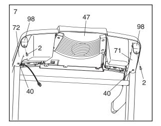
8. Touch the Right Handrail (72) to discharge any static. Insert the end of the Upright Wire (42) into the socket in the bottom of the Console Base (47). The connector should slide easily into the socket and snap into place. If the connector does not slide easily and snap into place, turn the connector and then insert it.
